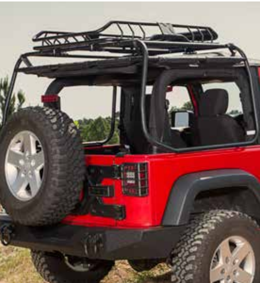
Use the optional Roof Rack Adapters to mount cross bars.
