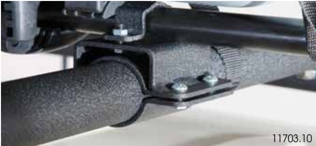
Use the optional Roof Rack Adapters to mount cross bars.
