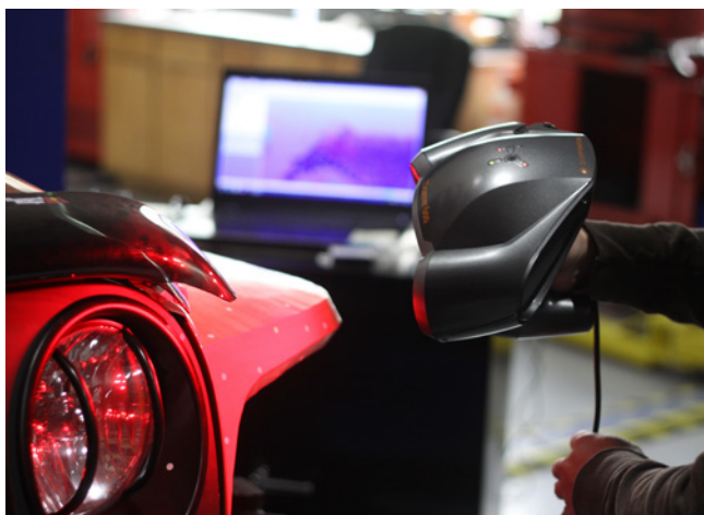
3D scan of clay model for CAD refinements.
