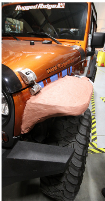
The process continues using clay, hand modeled directly on the body.
