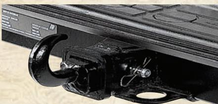
Heavy-duty black powder coated tow hook inserts into any 2" style hitch (does not include hitch pin, not designed for towing).
