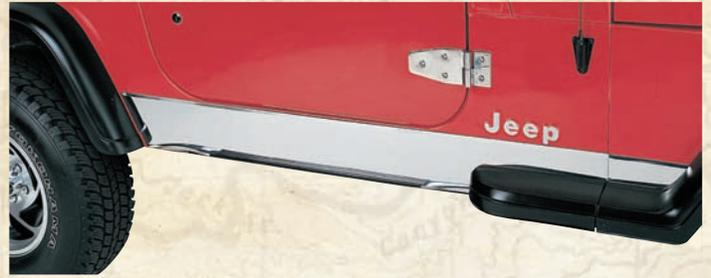
Made of highly polished stainless steel, these rocker panels extend from the front fender to the back fender. No drilling is required.
